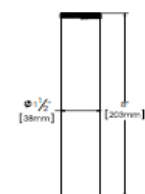
Fine Thread Tailpiece Attaches to 314 Series Direct/Offset Bath Wastes and Integral Bath Wastes.
